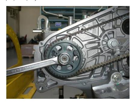
6 Set the extractor tool p/n 1860854000 to the drive pulley as shown in figure below
