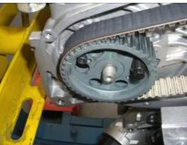
5 Undo the pressure pump drive pulley nut
