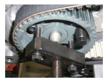
7 Rotating clockwise the screw on the extractor remove the pump from the mounting.
